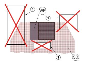
Figure: Safe distances from heat pump
