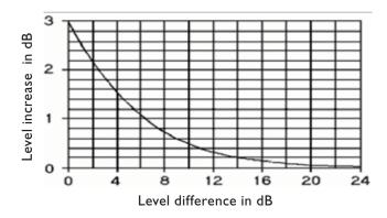
Example: If the level difference between two unequal sound sources is 5 dB, the level increase is an additional 1.2 dB.
