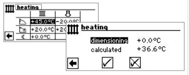
Menu line "dimensioning" Menu line "calculated" regional standard design temperature Calculated temperature heating curve
