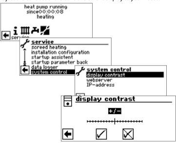
Adjust the contrast by turning the "rotary pushbutton"
