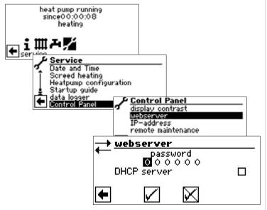
The screen switches to the "Web server" menu. Start by entering the 6-digit numeric password to unlock data input access. You will need this password later to register the computer with the controller. If you enter an incorrect numeric password, you will only be able to read data, but not make any changes.
