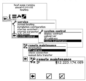
Enter the IP address of the remote maintenance server here (currently: 212.223.174.089)
