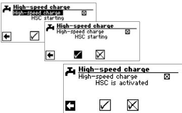
The high-speed charging is terminated analogous via the menu field "Terminate HSC SW":
