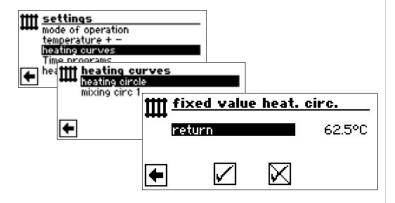
If the option "Fixed temperature" is switched on by the system setting, the screen changes to the menu "Heating curves" (which can take you to the menus "Fixed value heating circle" or "Fixed value mixing circle") or directly to the menu "Fixed value heating circle".
