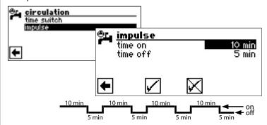
If the "Time off" setting is set to 0 minutes, the circulation pump will be switched on permanently during the released time periods.
