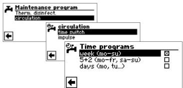
Use the time programs to specify the times during which the circulation pump is to run.
