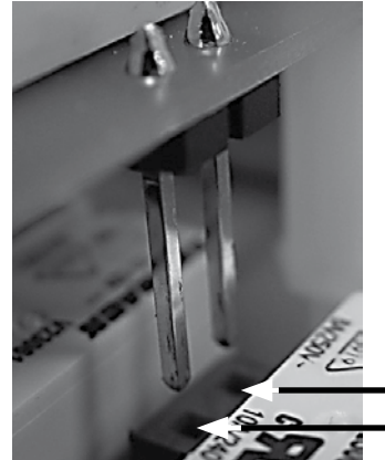
Socket (2) for upper contact pins of the Comfort board 2.0
