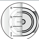
Measure the thread diameter (must measure 30mm)
